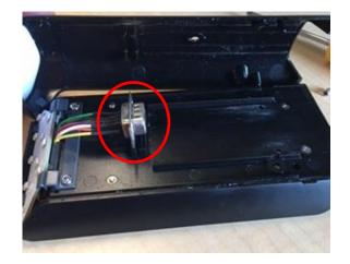
4. Put the back cover into the display port slot, but do not push the cover down.
