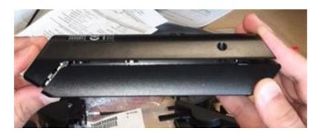
6. Reinstall the two screws in the back cover, and then reattach the console to the unit.
